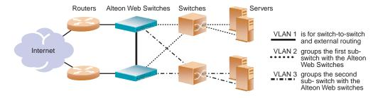
Figure 11-13 Using VLANs to Create Non-Looping Topologies
